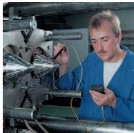
Fast surface measurements on plastic toolings (Probe 6910-0014)
