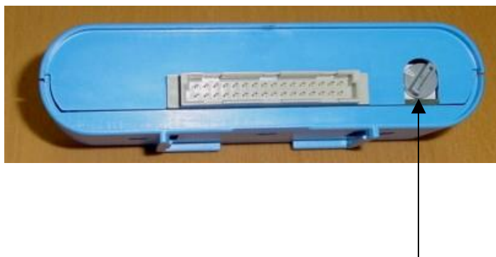
Rotary switch to set up TC
