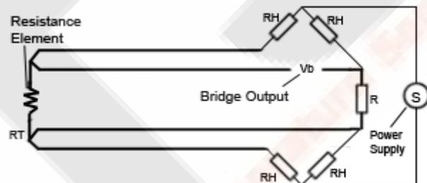
**Figure 3.** Lead wires have resistance that is a function of the material used, wire size, and lead length. This resistance can add to the measured RTD resistance, and improper wire compensation can result in significant errors. The common configurations of RTDs are two (A), three (B), or four wires (C).
