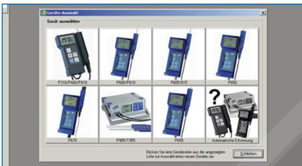
Automatic instrument- and port-identification
