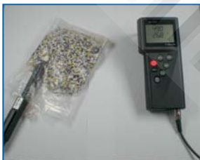
Measures equilibrium moisture in masonry, cement, plastic granulate
