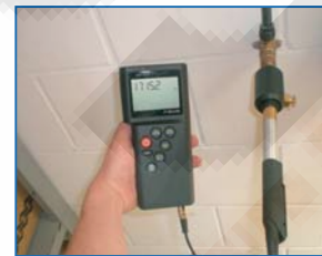
Pressure-tight moisture probe for measuring in compressed air
