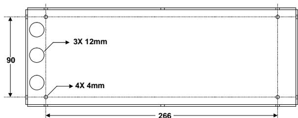
Figure 2 - Mounting the indicator in the panel cut-out.
